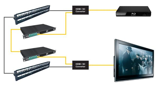
Connections between converters using multi-mode fiber optics and twisted pair cables
