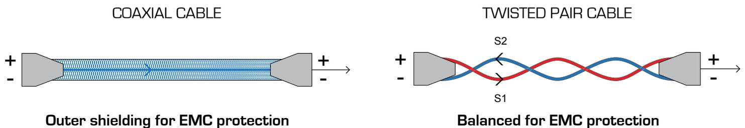
Given today's throughputs, a non-shielded twisted pair cable would seem to be an effective response to bandwidth requirements. The arrival of the 1000 BASE T and, in particular, the 10G BASE T with more sensitive encoding will lead to us favouring shielded options.
