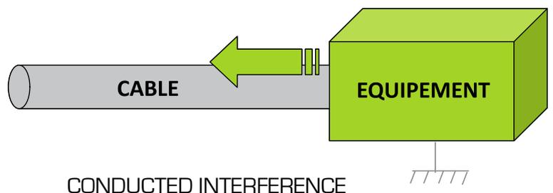
This interference is a characteristic of inductive or capacitive electrical phenomena associated with the performance of the products used and the quality of a system's installation. Regulatory documents are available on this topic which govern the entire scope of EMC
